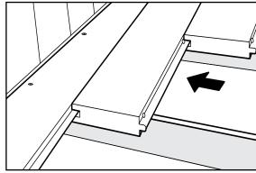
Note: Always follow best workmanship practices. Including, and not limited to, square cutting both board ends prior to installation.
