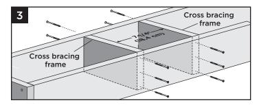
3. Install two 2" x 8" (5.1 cm x 20.3 cm) cross bracing frames in between joists at 7-1/4" (18.4 cm). Attach a total of twelve 3" (7.6 cm) pressure-treated compatible screws (not provided).
