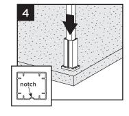
5. Attach bottom guide block using one 10 x 1" (25 mm) self-tapping screw (provided) in notch to lock guide block onto post.
