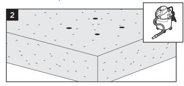
2. Clean out holes to remove all concrete dust.
