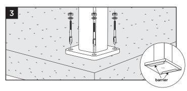
Insert (2) stainless steel barrier strips (not provided) under mounting bolt holes (these can be purchased on ShopTrex.com). Use appropriate shims if posts are not plumb. Secure post mount with the four expansion anchors, washers and nuts.
