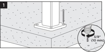
Using post as a template, mark locations of the four holes and drill into concrete at least 2-5/8" (66.7 mm) using a 3/8" (10 mm) masonry bit.
